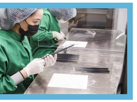
Numerous requirements are placed on the coating of these surgical tweezers: They should be elastic, have good adhesion, be free of cavities and be dirt-repellent.
