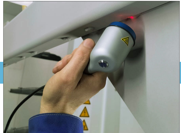
The PaintChecker mobile from OptiSense measures in even the smallest corner
