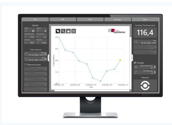
The OS Manager can also assess measured values directly as a line diagram. On the right, the important key data of the measurement can be read clearly and at a glance. Bild: Optisense
